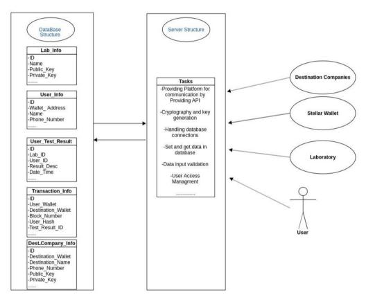
Fig 2. The system main components and data structure
